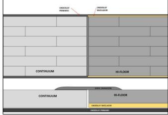
To achieve complete visual continuity of the two surfaces, we recommend an arrangement in which the panels are joined along their long sides. This ensures that the join between the panels using the clicking system is imperceptible.
