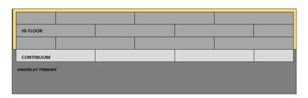
When attaching CONTINUUM BY FLINT panels to FLINT HI-FLOOR panels, make sure that the male and female elements fit correctly before applying tension. Failure to do so properly could result in damage to the CONTINUUM BY FLINT panel as it is made from a softer material than the FLINT HI-FLOOR. It is important to bear in mind that the floors have different degrees of hardness.
