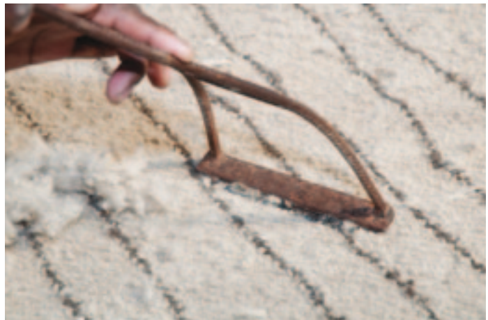
Brushing the pile to clean and to keep it softer
