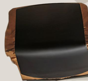
The impregnated substrates are stacked, pressed and cut into the Catifa Carta shell.
