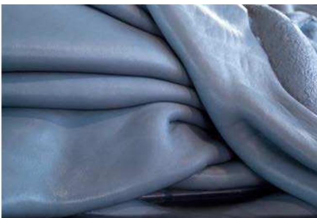
Leather tanned with chromium salts “ wet-blue ” and “ crust ”.
