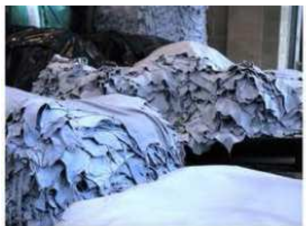
Leather tanned with chromium salts “ wet-blue ” and “ crust ”.
